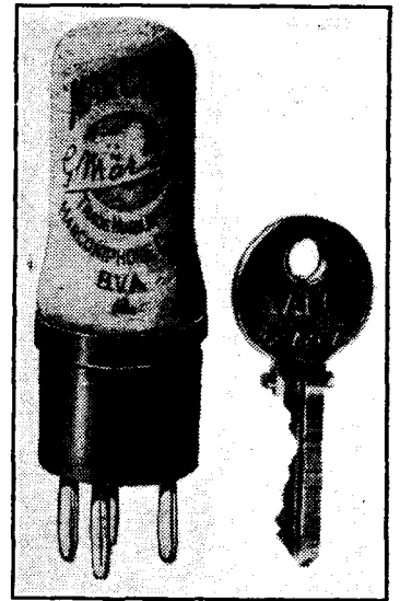
MIDGET VALVES FOR PORTABLES. The Marconiphone H.L.2 valve in the new "K" series. Its size can be gauged by comparison with the Yale key.
