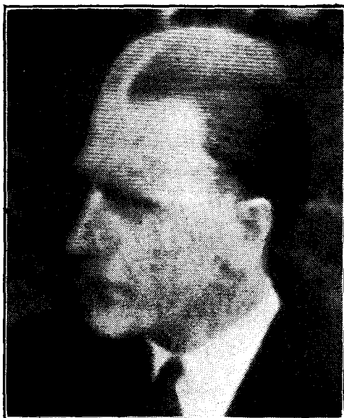
An untouched reproduction of a picture (of about 120 lines) from the receiver tube.
