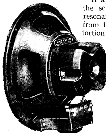
In the Celestion permanent-magnet loud speaker a wide air gap combined with an increased size of magnet gives freedom from fouling without reducing efficiency.
