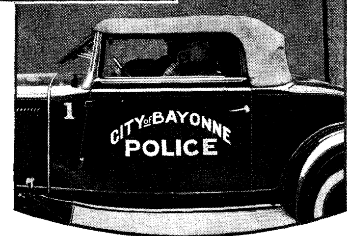
A typical patrol car. Note the plug-in microphone and antenna rod. (Inset) Bayonne's police chief at the headquarters transmitter.
