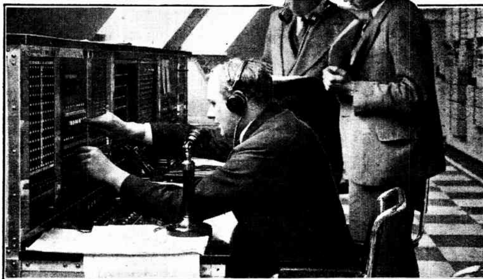
AT THE CENTRE OF AFFAIRS. All programme efforts in the studios, as well as all outside broadcasts, find their way to the control room at Broadcasting House, seen in the photograph. The engineer is seated at one of the S.B. desks.
