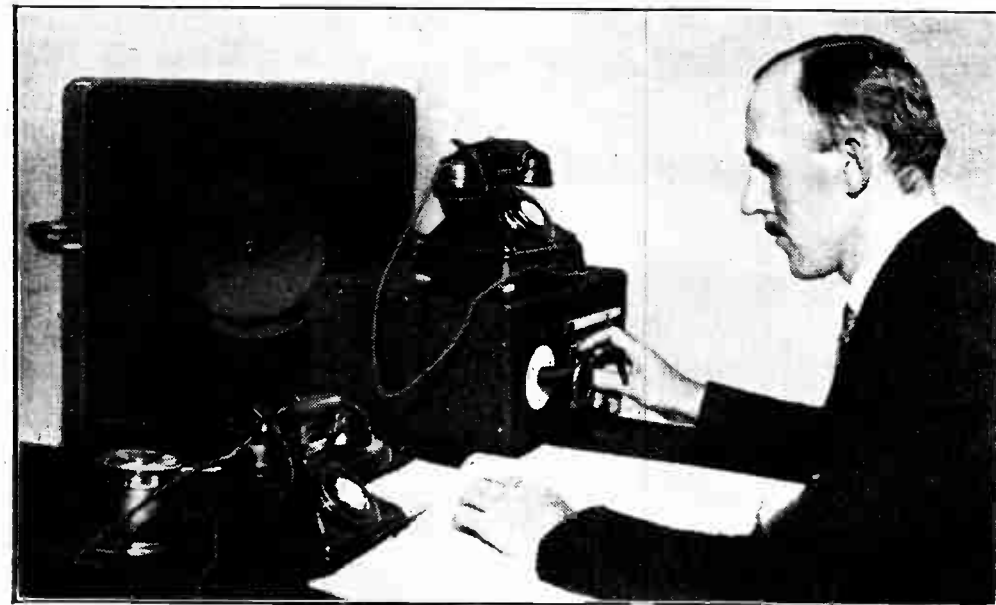
WATCHING POINTS. A supervising engineer at Broadcasting House checking the quality of transmission through a loud speaker fed from a check receiver. Quality is sometimes judged direct from the transmission lines between London and Brookmans Park.
