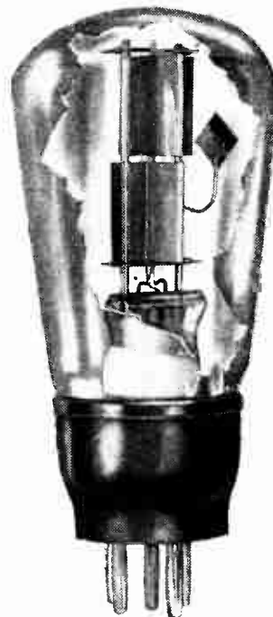
The Mazda AC/DD—the first British valve designed for full-wave detection and A.V.C. The bulb has been broken away to show the electrodes.
