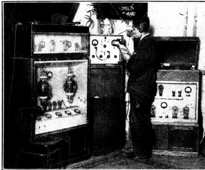
A CIRCUS SIDELIGHT. Tannoy public-address amplifiers supplying the giant loud speakers at Bertram Mills' Circus at Olympia. The \frac{1}{2} -kW. amplifier on the left delivers 180 watts of undistorted power and is used both for announcements and the relaying of bands.
