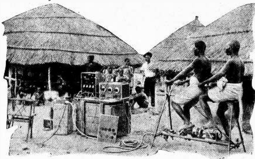
TWO-MAN-POWER STATION. One of a number of short-wave stations installed in isolated parts of Northern Rhodesia by the Marconi Company. The natives thoroughly enjoy the healthy exercise of generating the necessary 140 watts of electrical energy. Wavelengths of 40 to 60 metres are used.
