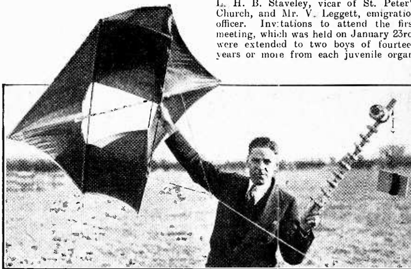
THE KITE SET. An official at the Radio Research Board's experimental station at Slough with one of the transmitter-equipped kites used for direction-finding tests. The padded valve is in the container at the end of the stick carrying the battery cells.
