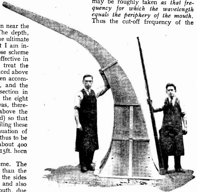
Fig. 2.—Metal portions of experimental 25ft. horn showing on the right the initial straight section which is 8ft. in length.
