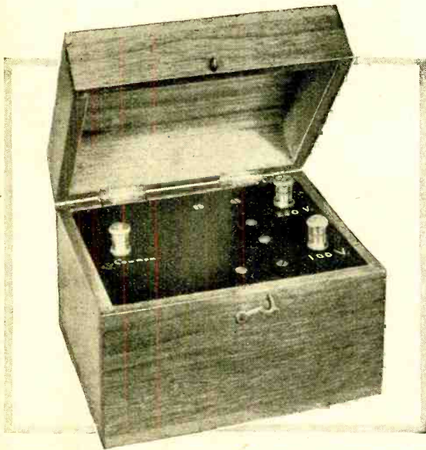
A separate voltage range box. Commercial power resistances in series with small home-constructed resistances are used.
