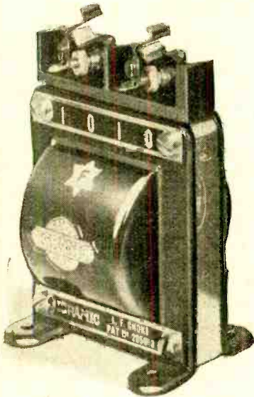
Igranic Type "F" choke with series-parallel connections.
