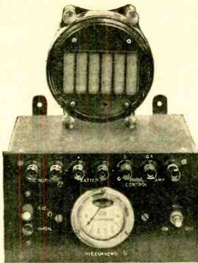
Igranic transverse current microphone and control unit.
