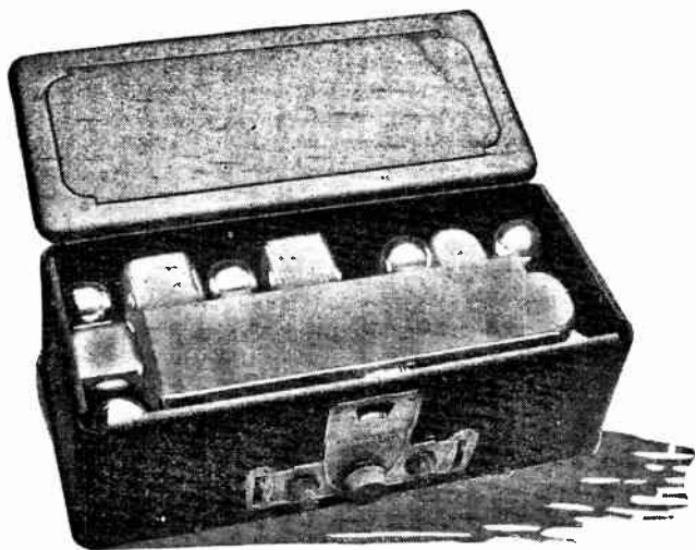
Progress in receiver design as illustrated in this compact six-valve set—the Rothermel-Crossley Band Box.
