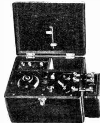
Bower-Lowe Mark II. Buzzer Wavemeter for wavelengths between 150 and 2,000 metres.
