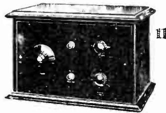
The B.T.H. 3-Valve Resistor Receiver. An extremely efficient receiver, employing resistance coupling, which gives perfect loud speaker results. It employs B.T.H. B8 Valves in the detector and first L.F. stage and a B.T.H. B 23 in the power stage. Changing from low to high wave lengths is carried out by a simple movement of a switch—no coil changing.
