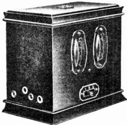
An example of German mass production methods: the Telefunken three-valve set which includes only two soldered connections and sells for the equivalent of £2 15s.
