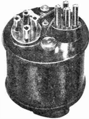
Gottlieb's Xiratone double-valve filament, whereby an extra stage of L.F. can be added without alteration to wiring.
