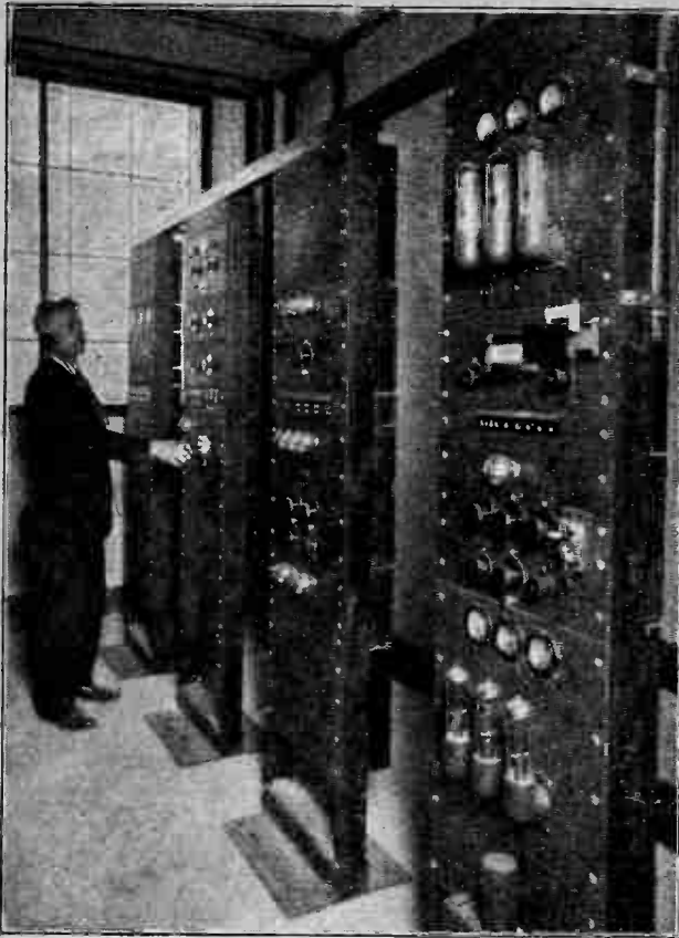
Fig. 3.—Low-power section of the transmitter, including speech input, modulating filter, and 750-watt amplifier panels.
