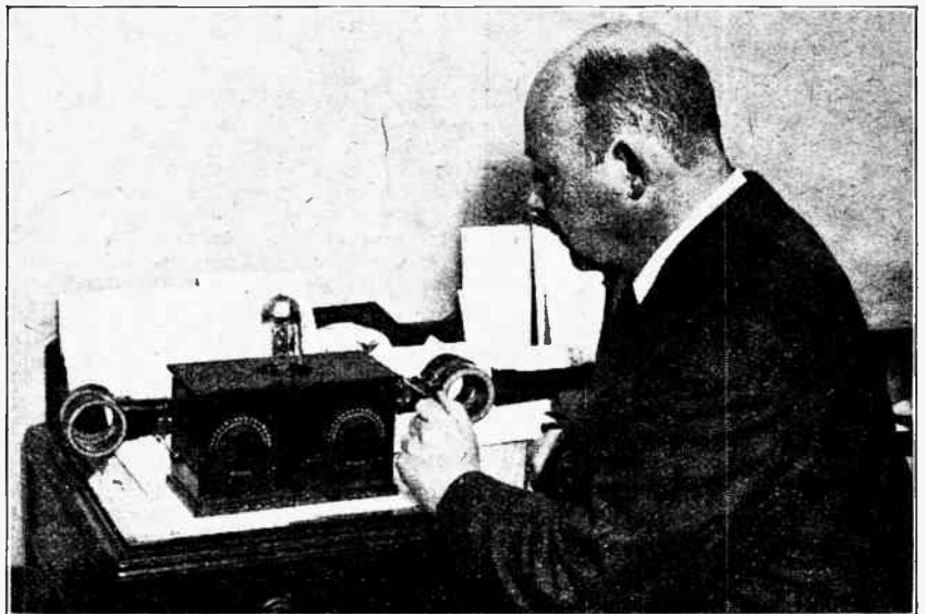
THREE VALVES IN ONE. A German inventor, Herr D. L. Loewe, is here seen with the remarkable valve which he has recently perfected. The valve incorporates a detector and both high and low frequency stages. Only a tuning unit is necessary to form a complete receiver.
