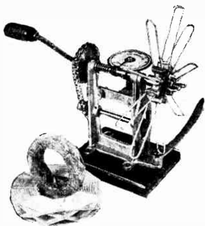
Kaynite duplex coil winding machine with examples of the type o. coil produced.
