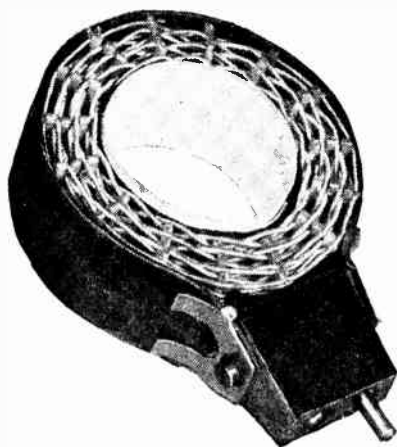
Multilayer coil of stranded wire. Inside diameter, 2in.; outside diameter, 3 1/8in.; length, 1 1/8in. Inductance, 115 microhenries; resistance, 4.5 ohms.
