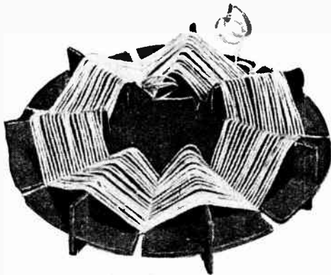
A cardboard former is used, and the construction will be seen from the illustration. There are 40 turns of No. 27 D.C.C. Inside diameter, 1 1/2 in.; outside diameter, 3 1/8 in.; inductance, 88 microhenries; resistance, 3.1 ohms.
