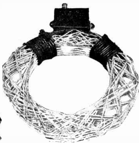
Multilayer coil of No. 22 D.C.C. Inside diameter, 2 3/4in.; outside diameter, 4 1/4in.; inductance, 131 microhenries; resistance, 4.2 ohms.
