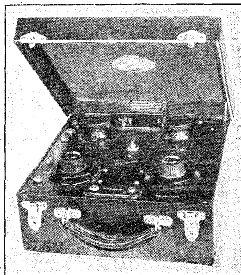
(Left) The "Pelican" uses a frame with oscillating detector valve and two stages of low-frequency amplification. (Right) Batteries and other equipment for the "Silvertone" receiver are carried in a separate case. A detector valve with variable reaction is fitted, followed by a single low-frequency stage. The instrument panel is of aluminium.
