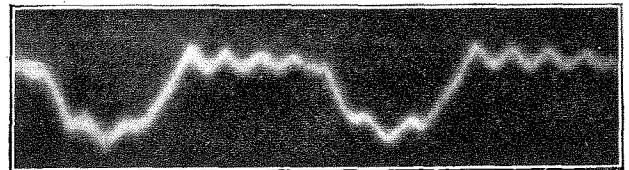
(F) This curve was taken when the valve had much too small a negative grid bias, and shows the waveshape of the current in the output circuit when the input current contained one harmonic.
