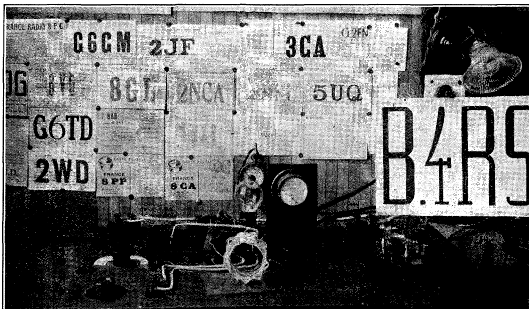
A well-known Belgian amateur transmitting station (4 RS), is extremely active, as may be judged from the "QSL" cards. His aerial consists of a twelve-wire cage, 160 feet long and 60 feet high.
