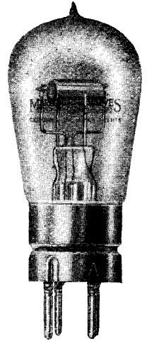
The D.E.R. Valve. The D.E.6 is similar in external appearance.
