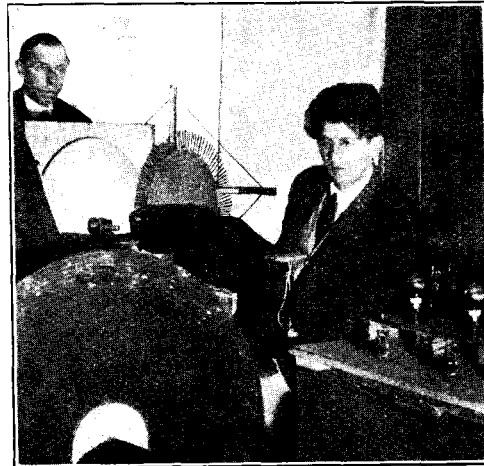
A photograph showing the transmitting apparatus, comprising the perforated disc, the disc with serrated edge and the selenium cell.
