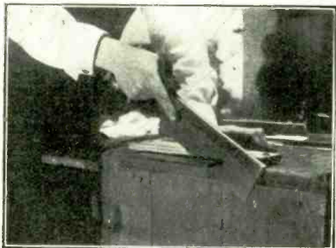
Fig. 5. The panel is secured to the bench for sawing off.
