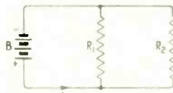
Fig. 10. This is a parallel circuit. The resistances R_1 and R_2 are connected in parallel. The effective resistance of R_1 and R_2 is less than either of them.
