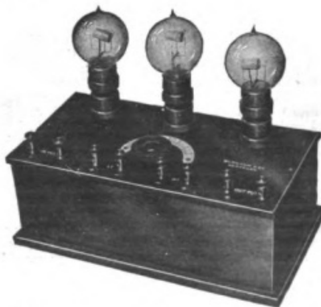
The photograph illustrates the three-valve, low frequency amplifier which Messrs. Burnham and Company are awarding to Mr. Wade.
