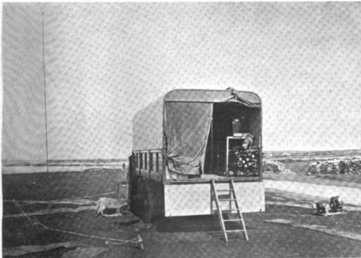
A motor lorry used for demonstrations of wireless in a tour round the country. Note the 70-ft. portable mast, the earth-mats, and the engine generator on the right.
