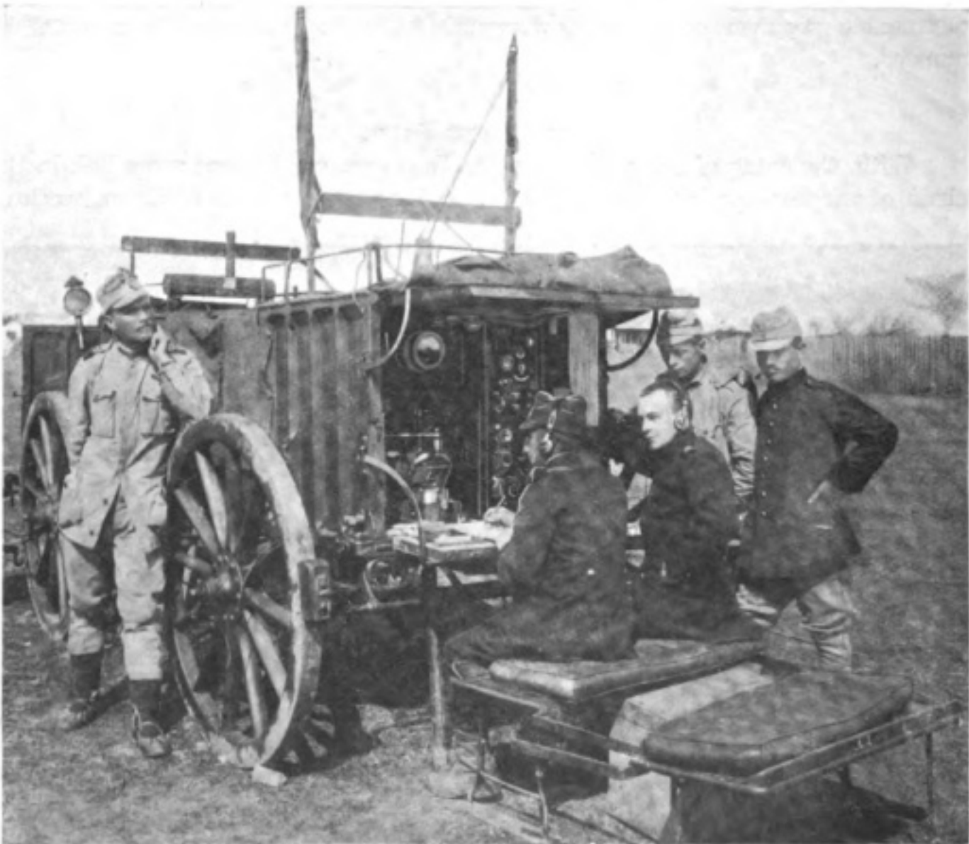
TWO PHOTOGRAPHS OF ROUMANIAN FIELD WIRELESS STATIONS. ABOVE, THE ARRANGEMENT OF THE PORTABLE MASTS AND THE APPARATUS CART CAN BE SEEN ; BELOW, ROUMANIAN OPERATORS (ONE WITH HIS CAP ON !) ARE SEEN WEARING THE TELEPHONES AND RECEIVING MESSAGES FROM A DISTANT STATION. NOTE THE COMPACTNESS OF THE APPARATUS (MARCONI SYSTEM).
