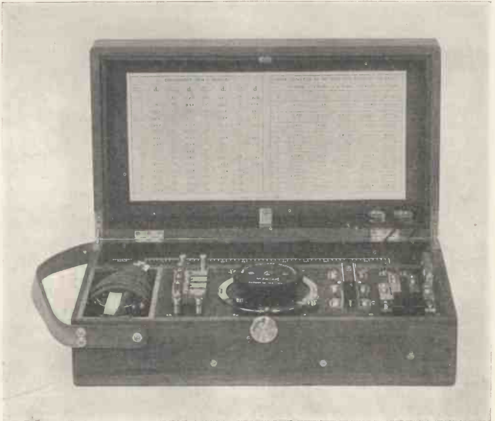
Marconi Direct-reading Portable Decremeter.
