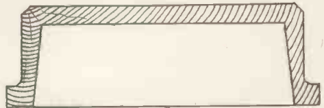
SECTION OF PATTERN FOR ALUMINIUM CASE.
