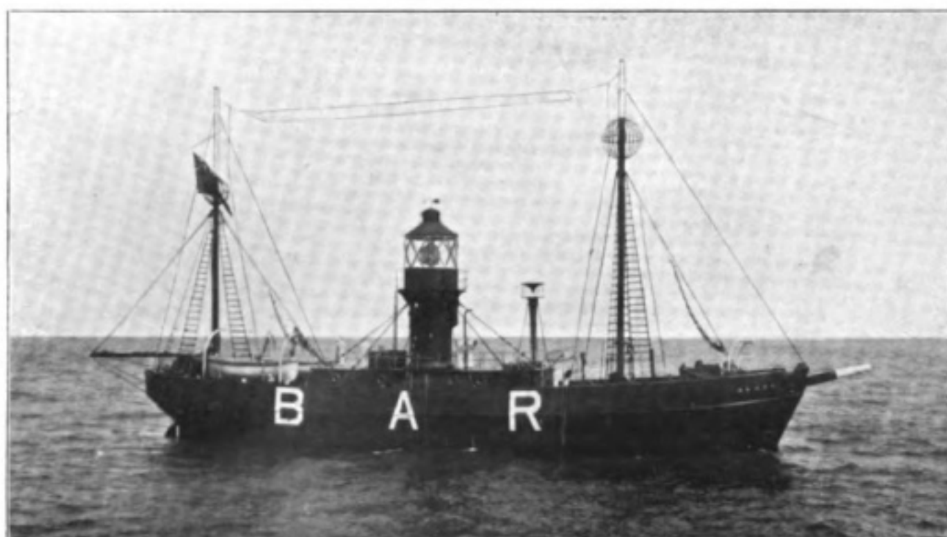
The New Lightship "ALARM" now in position on the Mersey Bar Station. She has a light of 40,000 candle-power and is fitted with a Wireless Installation and a Submarine Bell. A Wireless Installation has also been erected at the Dock Office to place both the Bar and the Formby Lightship in communication with the Dock Office Building.
