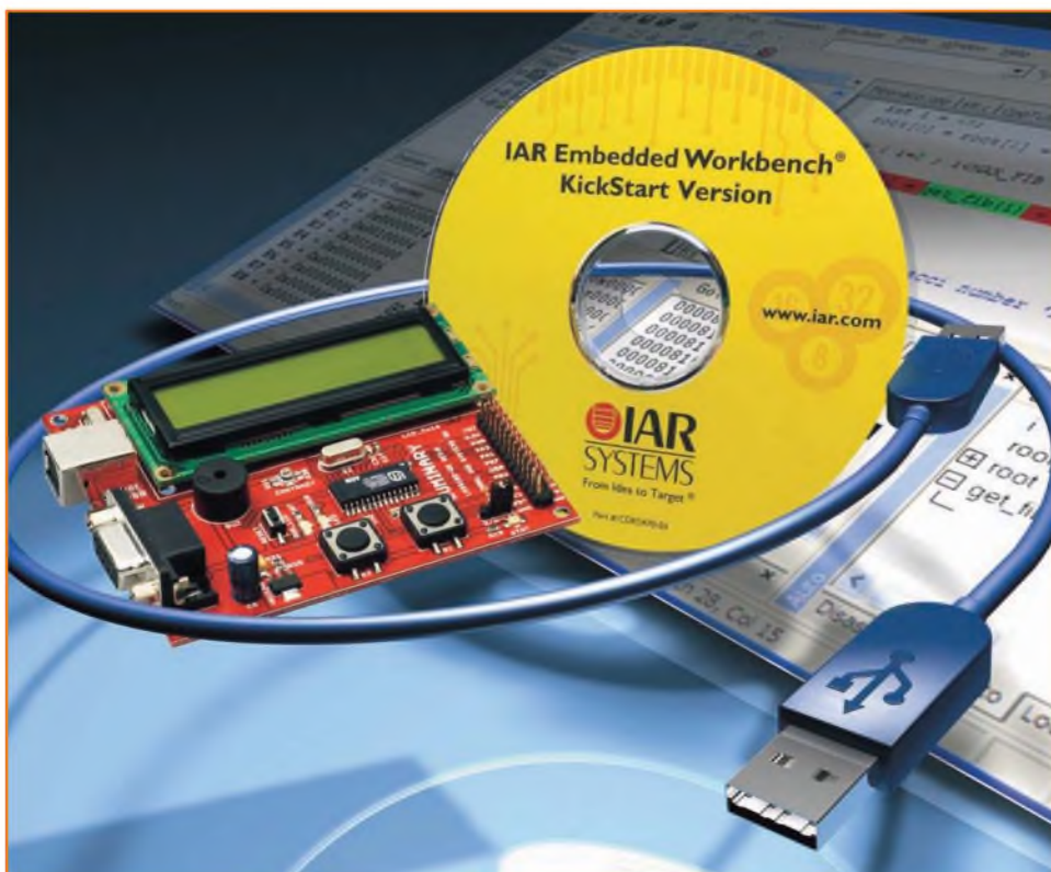
Figure 1: Luminary Micro introduced the first Cortex-M3 based microcontroller for less than $1, shown here on an evaluation board as part of an IAR KickStart Kit
