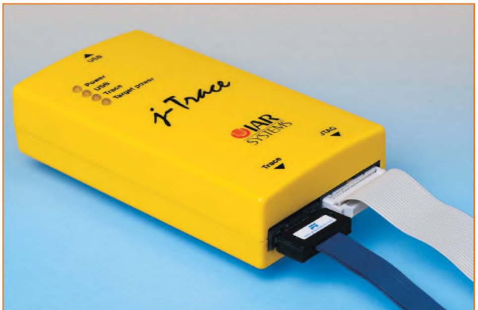
Figure 2: Embedded Trace Macrocell makes it possible to carry out a wide range of debug and monitoring functions within the core
