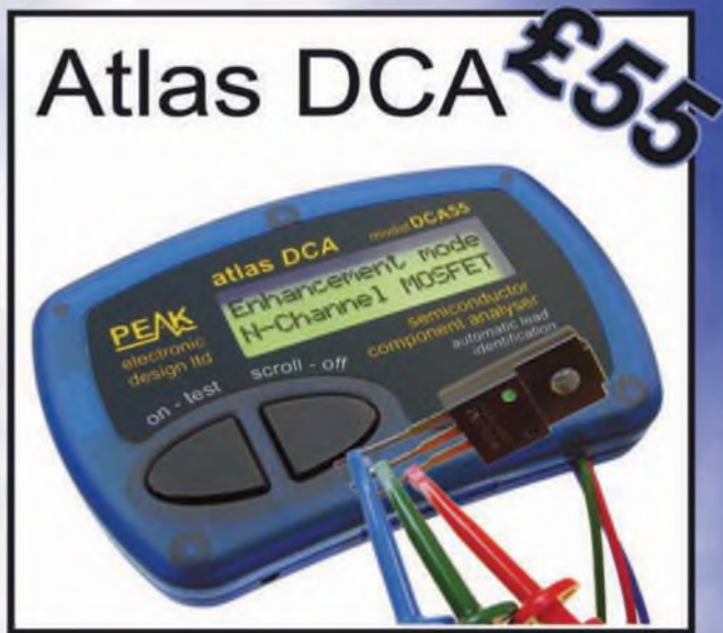
Atlas DCA - Model DCA55 Semiconductor Analyser
