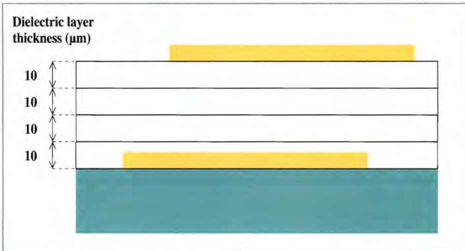
Figure 8: Printing four layers of dielectric paste to achieve a total fired thickness of 40µm
