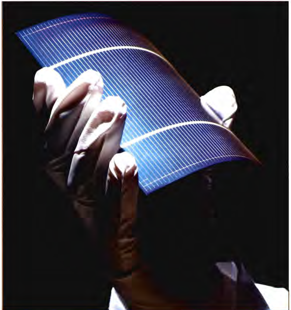
Large area i -PERC solar cell on a very thin wafer
