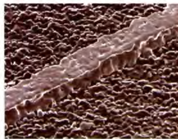
Figure 1: Photographs of 20µm wide conductor tracks formed using the HC4700 silver paste
