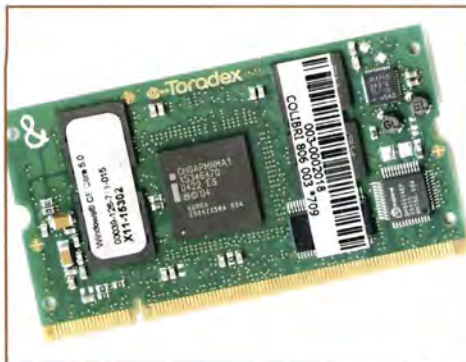
Prototype of a Marvell PXA320 SODIMM module for handheld devices
