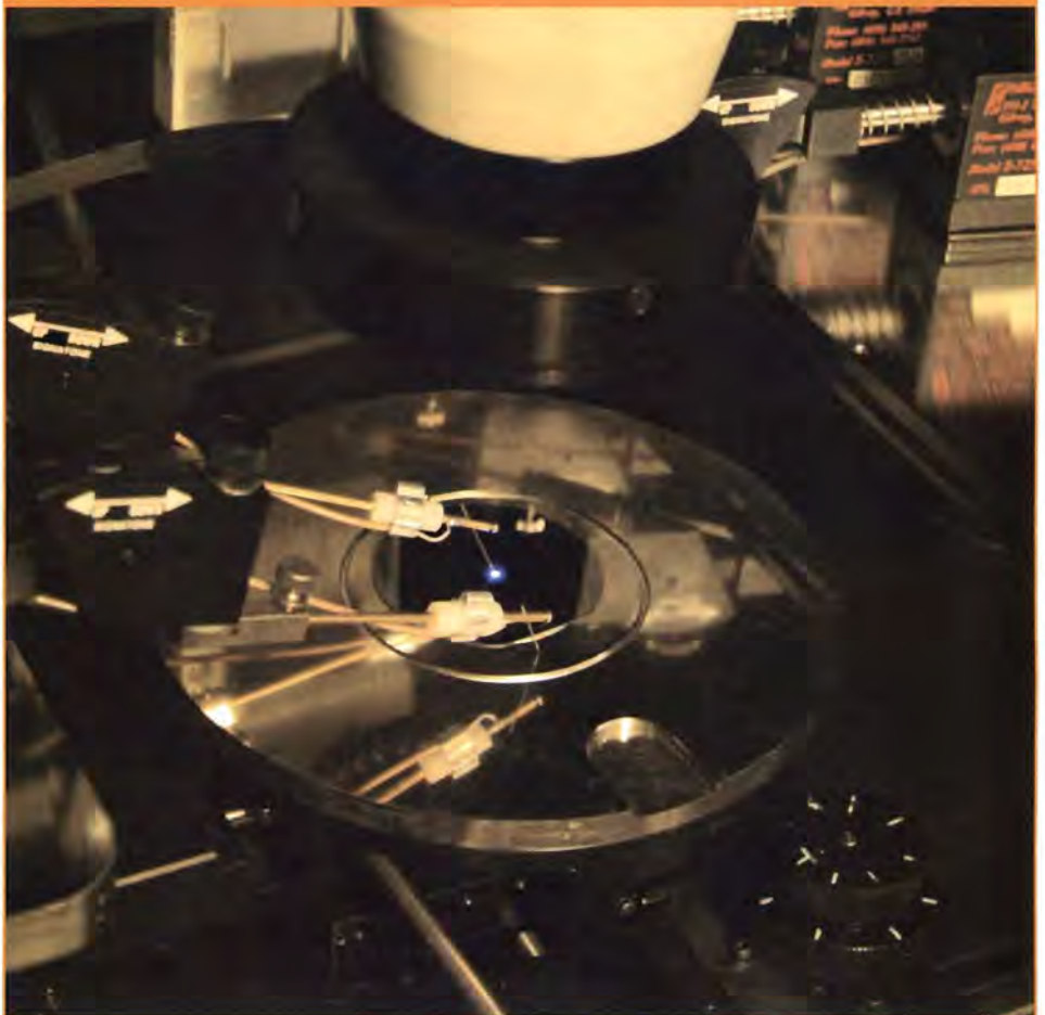
Figure 4: Prototype GaN LED grown on a silicon wafer being probe tested at the laboratory in Cambridge University
