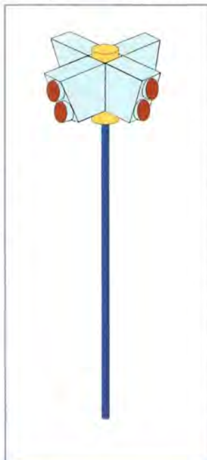
Figure 1: Millimetre microwave transceiver using fibre-optic system
