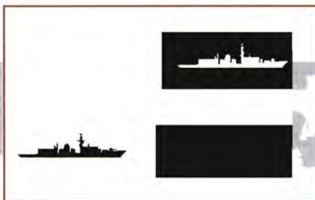
Figure 1: A simple example of how visual contrast is determined by the variation of the ship against its background
