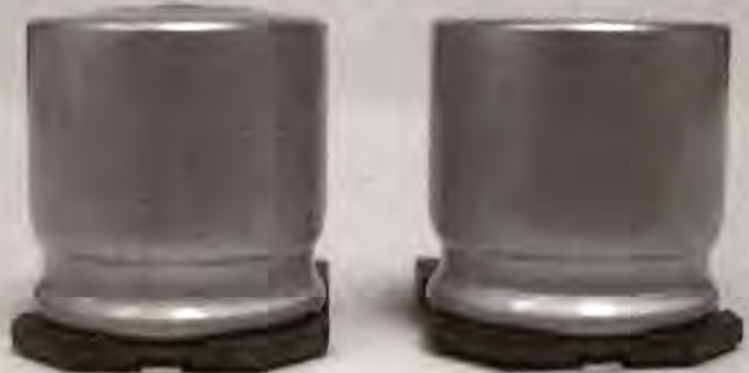
Figure 1: Aluminum liquid electrolytic capacitor, on the left-hand side, that has experienced case distortion after an extended time at Pb-free reflow temperatures
