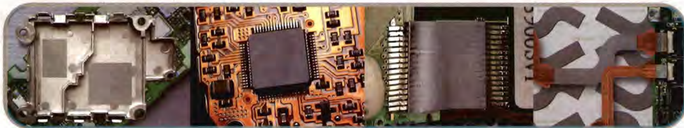
Figure 1: EM absorption using cut-to-shape Flexield from TDK, where Flexield is a flexible, thin ferrite based electromagnetic (EM) wave absorber material that can be cut to shape and attached to the interfering component or the shield can via its double sided adhesive
