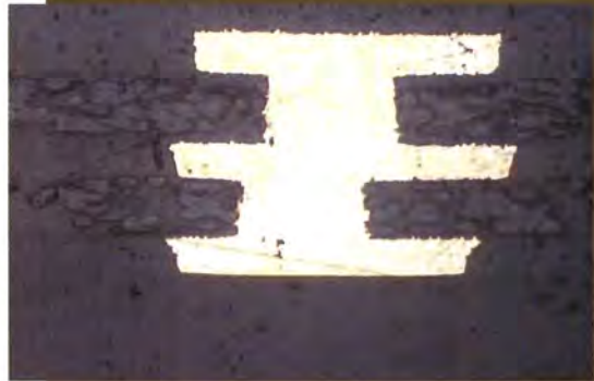
Figure 4: A 4+n+4 construction microvia tower, using a 125-micron laser drill (communications application)
