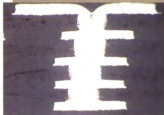
Figure 4: A 4+n+4 construction microvia tower, using a 125-micron laser drill (communications application)
