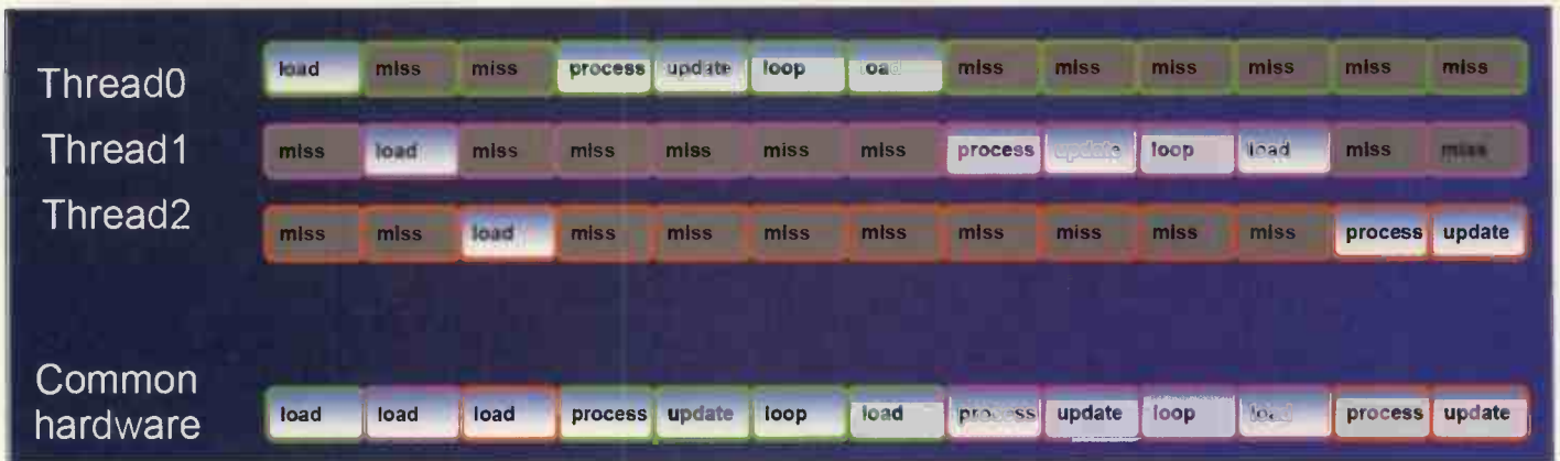
Figure 3: Improving pipeline efficiency with multiple threads
