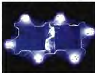
A part of a mesh module enabling the easy fabrication of a large area backlight unit for LCD screens, as prepared by Oree
