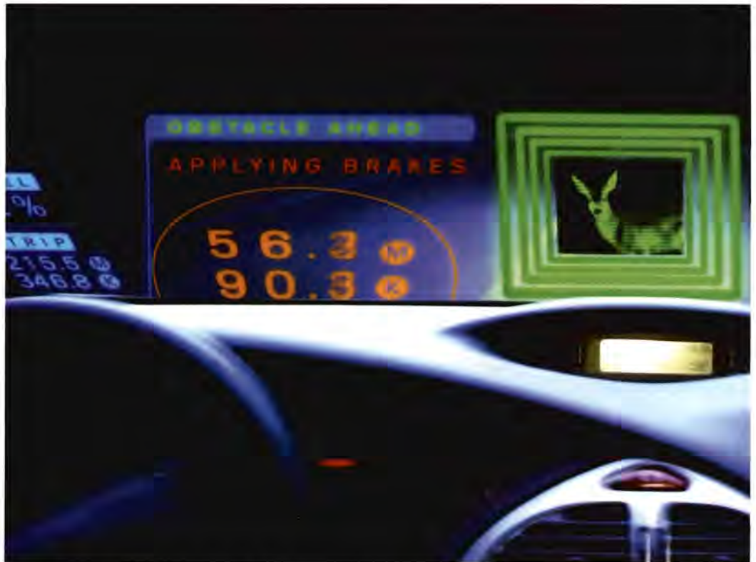
Potential automotive application for the DaVinci technology. A video image can be processed using a DSP camera providing a head-up display
