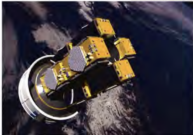
Between six and eight Galileo satellites could be launched on each Ariane 5
