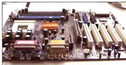
Figure 15: Elite K7S5A motherboard
