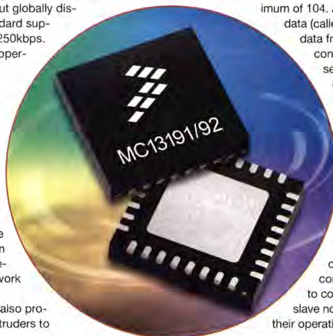
Figure 4: ZigBee chipset from Freescale Semiconductor
