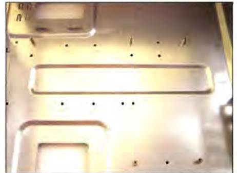
Figure 16: The standoffs for mounting the motherboard
