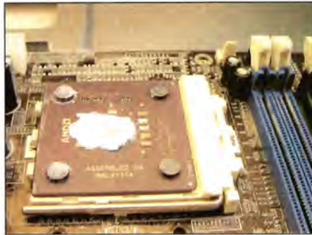
Figure 7: CPU in a ZIF socket with a visible white thermal paste
