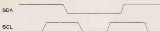
Fig. 2. The 'Transmission Start' sequence precedes every transmission of a command from the microcontroller to the SHT11 integrated sensor.
