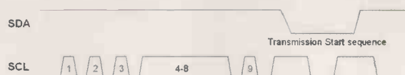
Fig. 3. If communication with the SHT11 device is lost a 'Connection Reset' sequence has to be issued from the microcontroller, which toggles the SCL line nine times or more.
