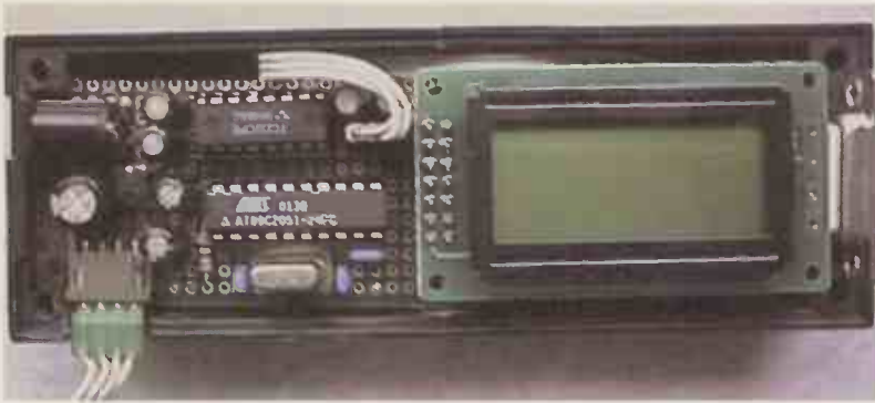
Fig. 7. Internals of the RHTS-11L device with the display mounted in a piggyback-style and the 89C2051 microcontroller in the middle.
