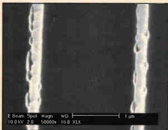
Microscope photos of low-k conductors subjected to ‘stress-free polishing’, left, and conventional polishing, right.
