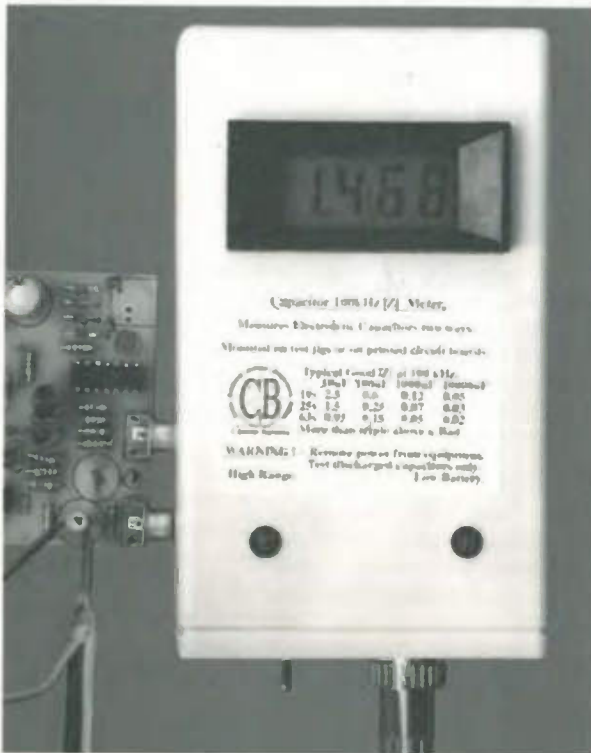
Fig. 2. Prototype meter performing an in-circuit measurement using my 'best' four-wire test-lead set.
