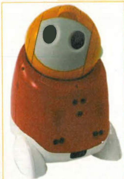
NEC has developed a personal robot called PaPeRo (partner-type personal robot) that can recognise 650 spoken phrases and speak more than 3000.
