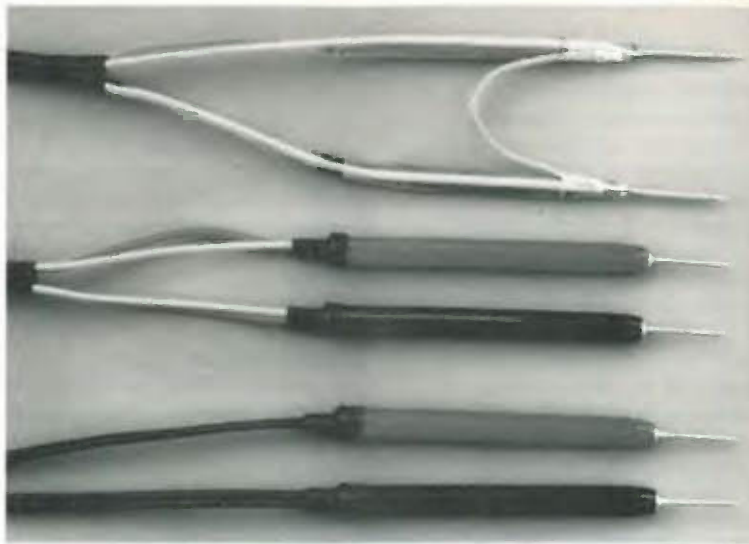
Fig. 7. This photo shows the test probe ends of the three test lead sets I assembled. The 'best' set, with its external braid link, can be seen at the top of the picture. The easiest to assemble lead was made using the black four-way screened flat strip cable at the bottom.
