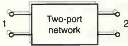
Fig. 2. The most common type of network has two ports and neither is strictly an input or an output.
