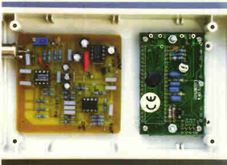
Fig. 3. This photograph illustrates one possible packaging option, in an OKW 'Shell' case, resulting in a battery powered, self contained, portable AC millivoltmeter. This case provides a removable aluminium front panel able to support a panel mounting BNC socket and on/off switch.
