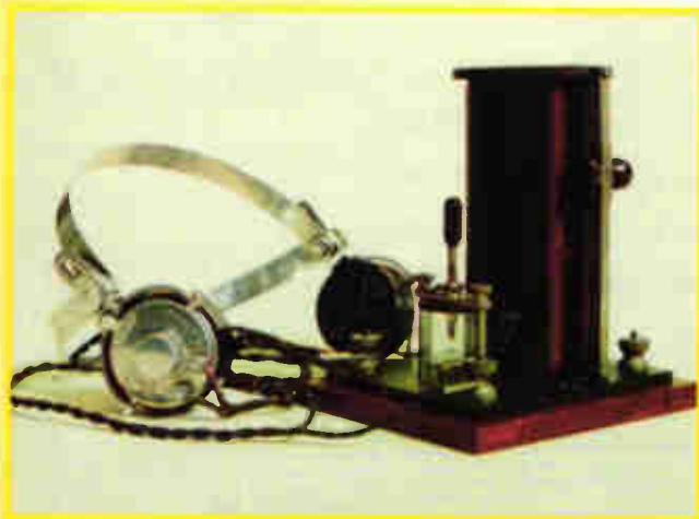
The once common crystal set. Available in the early 1920s, this version needed a long antenna.
