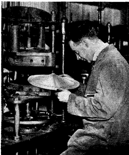
(Above) A high-speed machine winding energising coils for H.M.V. loudspeakers. (Left) The thick pulpy cone is subjected to a "blocking process" which reduces it to a closely woven material of the correct thickness and weight
