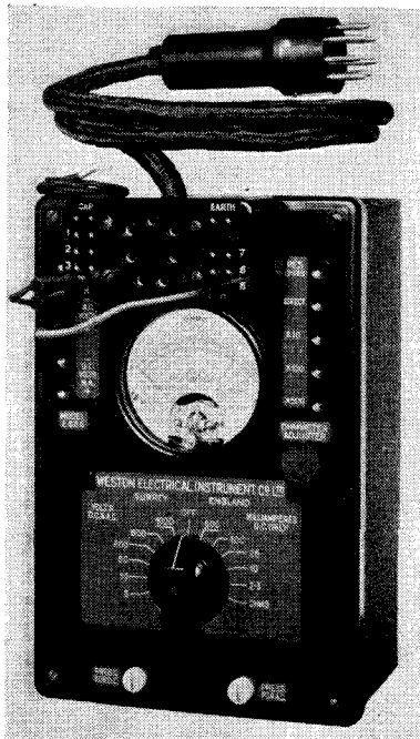
"... a habit guaranteed to ensure safety; make a rule to set the switch to the highest range before placing the meter in circuit."
