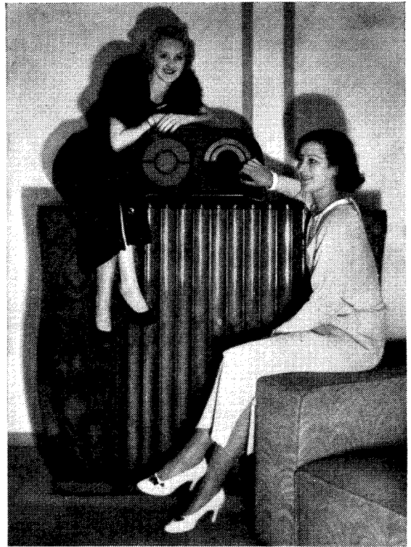
Two musically-minded maids with the "streamlined" Ekco AC86—a five-valve super for A.C. mains operation. The AC86 is a new season's set that does work well!
