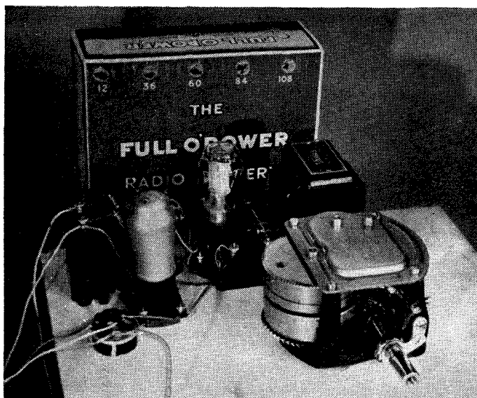
Inverted, the motor board is seen to carry all the parts, including valves. Constructional work is particularly simple.
