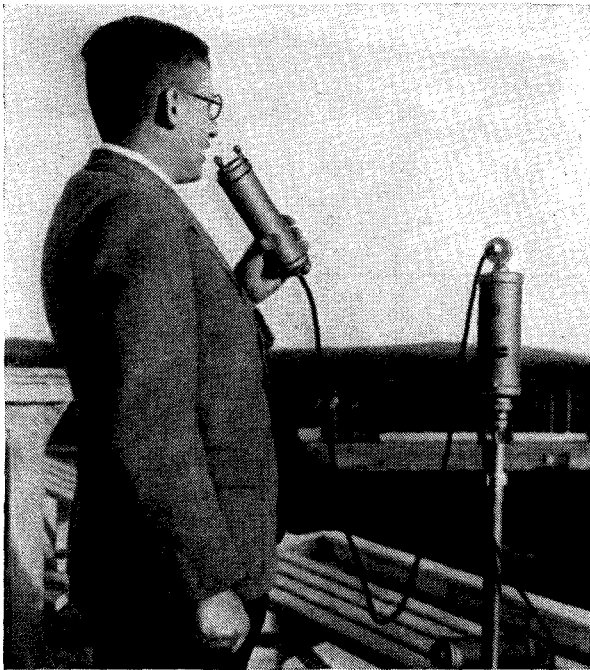
Crystal microphones are now being extensively used by the German broadcasting organisation. Here is one in use for the broadcast of a sports relay. Its comparative lack of sensitivity enables the commentator's voice to be distinctly heard without crowd-noise interference
