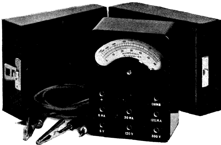
A combination meter like the invaluable "Avomator" in conjunction with a valve-base adaptor enables one to do a very systematic job of fault-tracing
