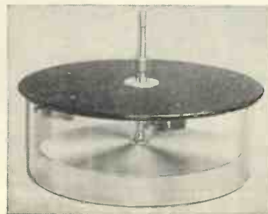
ADJUSTABLE GLASS ELECTRODE Another of the electrodes used by the inventor. It is made of glass and can be adjusted by the movable condenser disc
