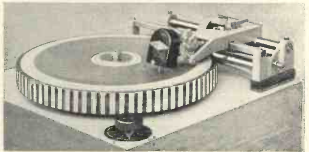
FOR DIRECT RECORDING ON DISC This new Parmeko direct-recording outfit is provided with a heavy turntable driven by a synchronous motor. It cuts perfect records that can be played many times with a steel needle
