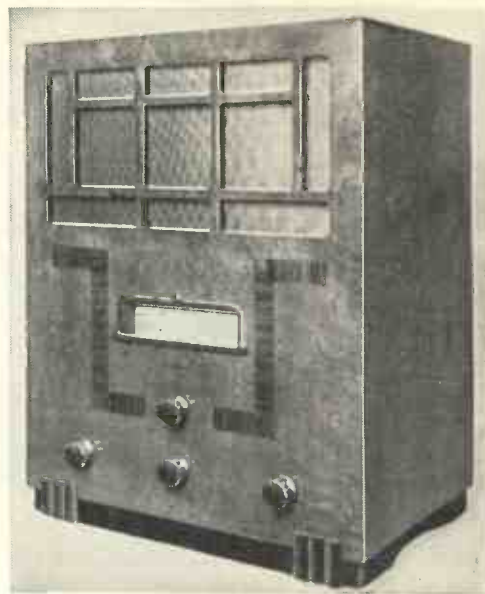
"Four controls are all you have to worry about, although there is a fifth which governs the set's sensitivity at the back of the chassis"
