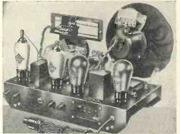
"Provision has been made for external loud-speakers, a gramophone pick-up, a power point to feed a gramophone motor or external reproducer"
