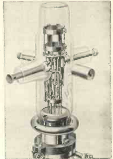
LARGE POWER VALVE A water-cooled high-power valve used in the output stage of ultra-short-wave therapy apparatus
