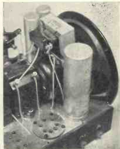
CLOSE-UP OF THE LOUD-SPEAKER The loud-speaker is mounted immediately behind the low-frequency choke. The necessary connections can be followed easily from this photograph
