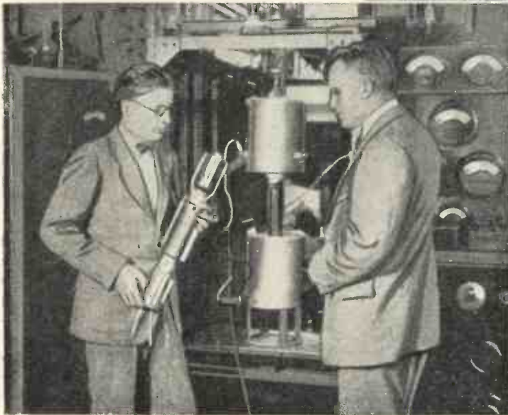
AT WORK IN THE LABORATORIES (Above) G. W. Elmen at work in the Bell Magnetic Laboratory where he has developed remarkable new magnetic alloys. (Left) Two of the Bell experts with a high-power water-cooled valve developed under their supervision for the Atlantic telephony service
