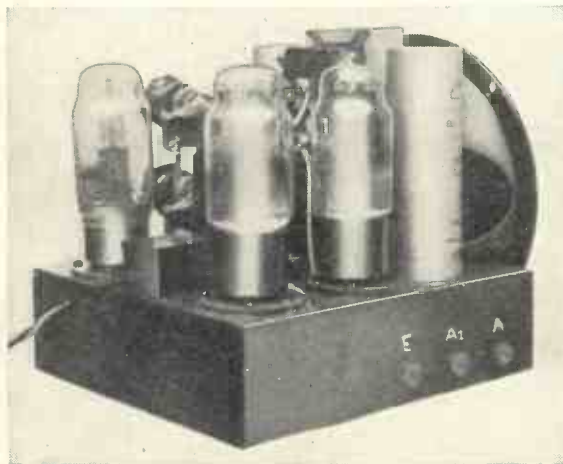
ALTERNATIVE AERIAL TAPPINGS The aerial and earth sockets are fixed on one side of the wooden baseboard assembly. The set will give good results from an indoor aerial if used in a Regional area
