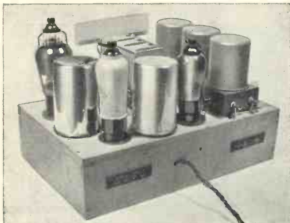
SIMPLE YET OUTSTANDING DESIGN A back view of the Heptode Super Three showing the set chassis ready for fitting in the cabinet. It is built up on a metallised wood chassis
