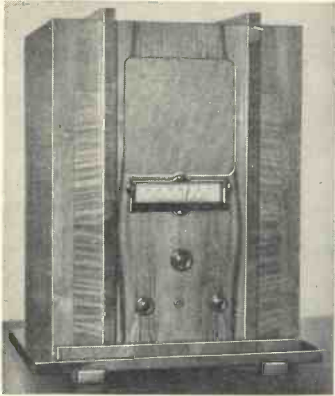
"It is suitable for A.C. or D.C. mains of any voltage with any A.C. frequency . . . simplicity of control is the salient feature"
