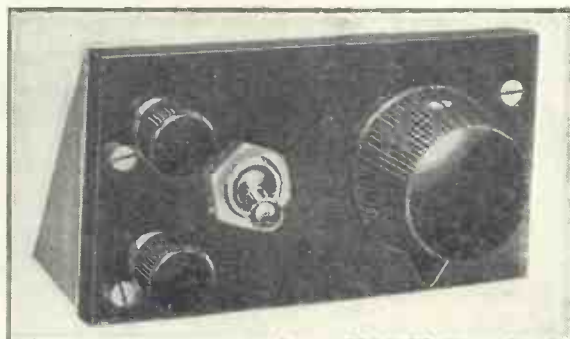
ADAPTOR UNIT FOR GRAMO-RADIO This unit is screwed to the back of the cabinet if it is required. It consists of a volume-control potentiometer and a gramophone switch
