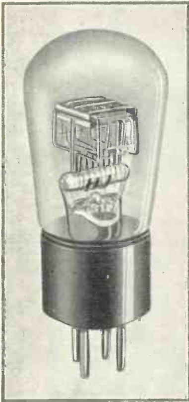
BATTERY SUPER-POWER VALVE This photograph shows the electrode arrangement of a Mullard PM202 super-power valve for battery operation
