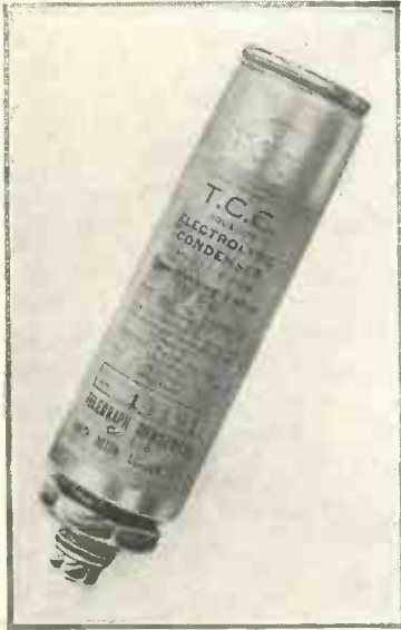
WITH AQUEOUS ELECTROLYTE This T.C.C. electrolytic condenser has a capacity of 8 microfarads, in spite of its small size
