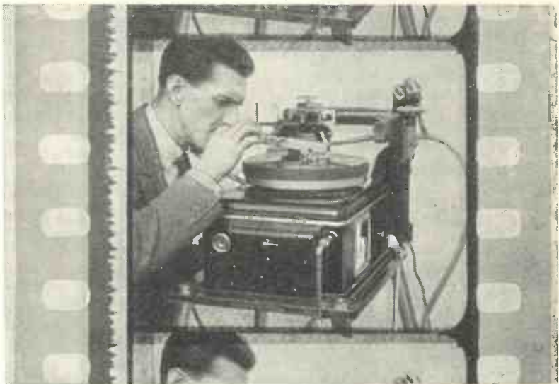
SAMPLE OF FILM MADE BY PATHÉ PICTURES Part of a sound film, showing H.M.V. disc recording in progress. On the left the R.C.A. type of variable-area sound track can be seen
