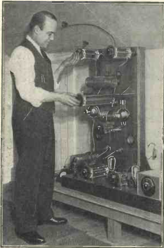
SOMETHING LIKE CONDENSERS! This photograph shows the apparatus used by an American amateur transmitter. He certainly has a unique collection of variable condensers for tuning
