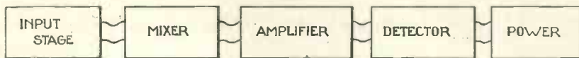
Fig. 1.—The five essential parts of a super-het set as exemplified by the Super 60 series
