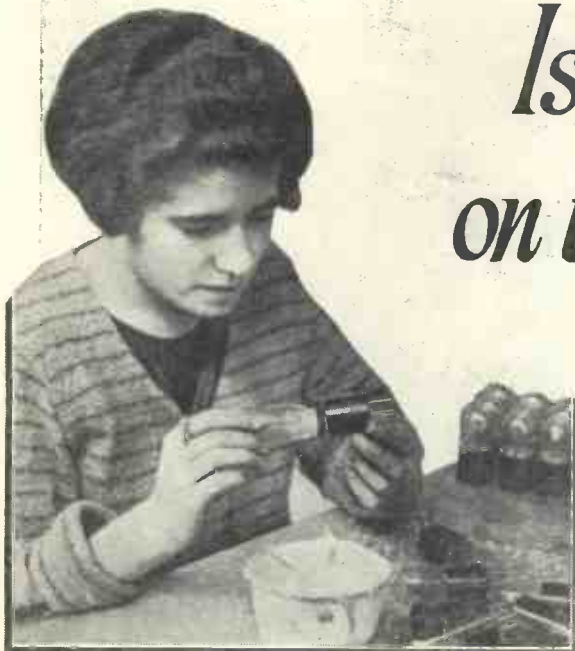
AN IMPORTANT PART OF VALVE MANUFACTURE This photograph shows how the glass bulb of a valve is fixed into the insulating base. The process is known technically as "capping"
