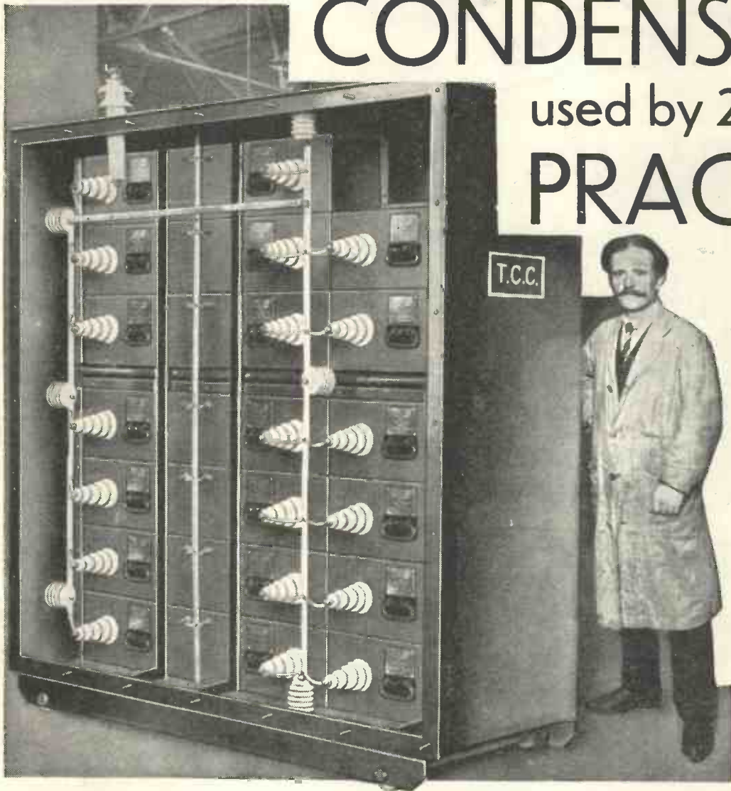
Here is illustrated one of the seven giant 5 mfd. condensors standing 6 ft. 6 ins. high.
