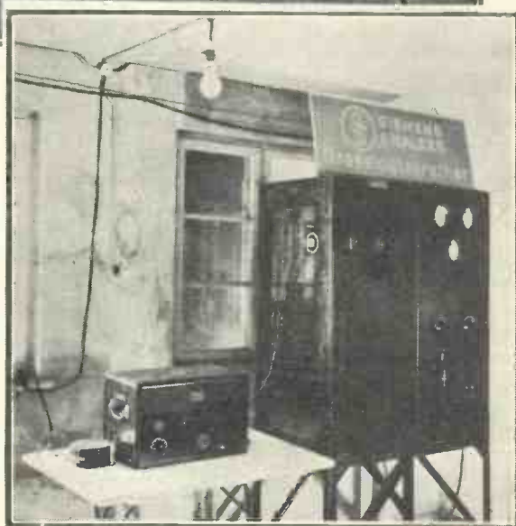
ONE OF THE 200-WATT AMPLIFIERS One of the 200-watt amplifiers made by the Siemens and Halske people for supplying power to the thirty-five loud-speakers at the Avus race track
