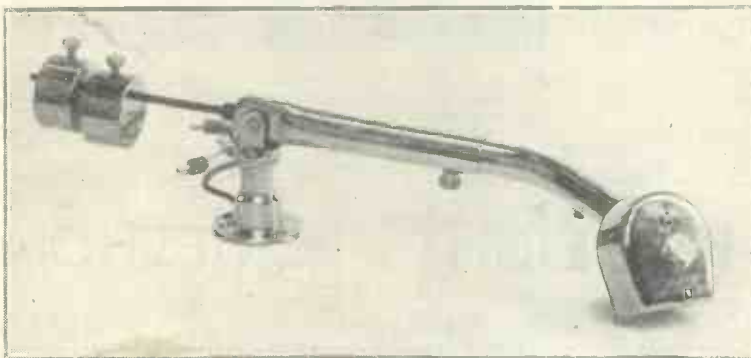
CAPTAIN BARNETT'S EXPERIMENTAL PICK-UP This is the B.T.H. Senior pick-up as adapted by Captain Barnett for his featherweighting experiments.
