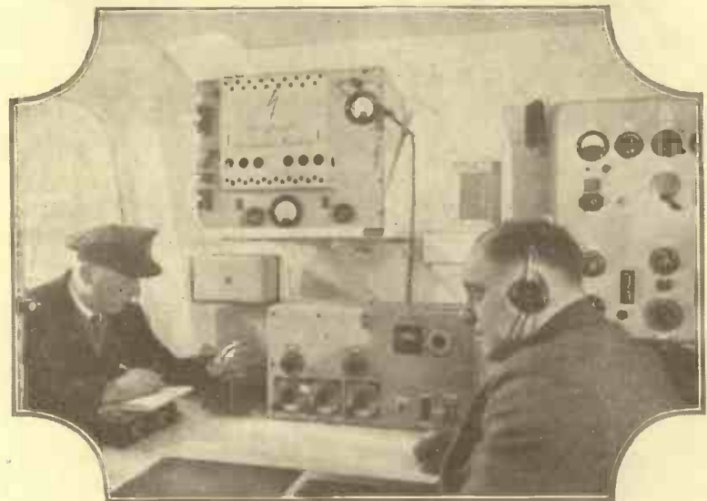
SHORT-WAVE TRANSMISSIONS FROM THE AIR An interesting photograph of the radio apparatus installed on the Graf Zeppelin. Quite short wavelengths are used for the transmissions
