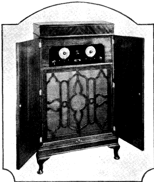
This photograph shows the complete A.C. Super 60, the radio gramophone that W. James uses at home. Note the fine appearance of the Osborn "Queen Anne" cabinet. The frame aerial is placed on a small bracket on the outside of the case
