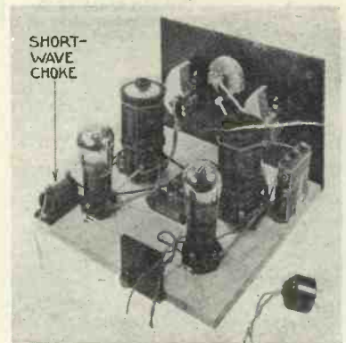
Here you see the adaptor ready for use with valves and coils in position. A plug on the unit is plugged into the set
