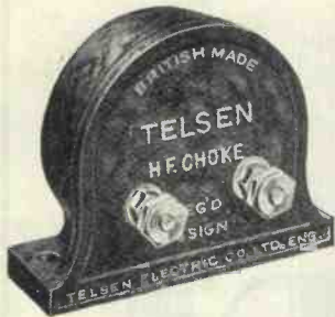
TELSEN H. F. CHOKES. Designed to cover the whole wave-band range, from 18 to 4,000 metres. Extremely low self-capacity, shrouded in Genuine Bakelite. Inductance 150,000 microhenries, resistance 400 ohms. Price 2/6 each.
