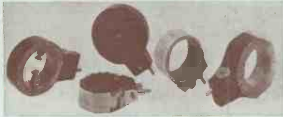
Five different makes of two-pin plug-in coil. That on the extreme left is of the X- or double-tapped types, used for obtaining increased selectivity
