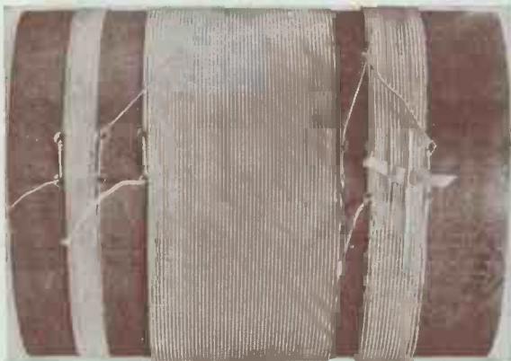
A single-layer or solenoid type of tuning coil. The photograph shows clearly how the wire is anchored by threading it through holes in the former
