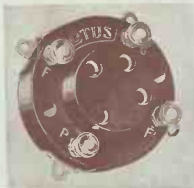
On this valve holder the letters F indicate the two filament sockets, G the grid socket, and P the plate or anode socket
