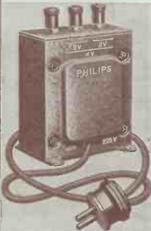
A.C. (alternating current) can be stepped up or down in voltage to any required value by means of a transformer. The type shown here is for supplying 4 volts to the filaments of mains valves
