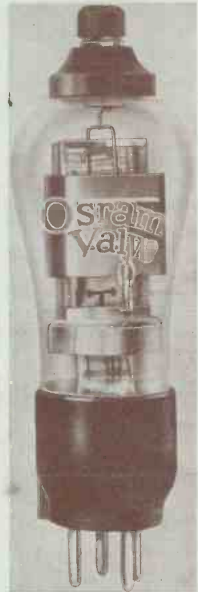
The modern type of screened-grid valve has an ordinary base, but there is a terminal at the top for the anode connection. Such valves are usually used in conjunction with external metal screens
