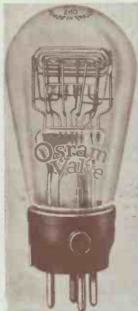
This pentode valve has five grids and gives enormous amplification. Only one extra connection is necessary. The terminal on the base is connected to the high-tension battery
