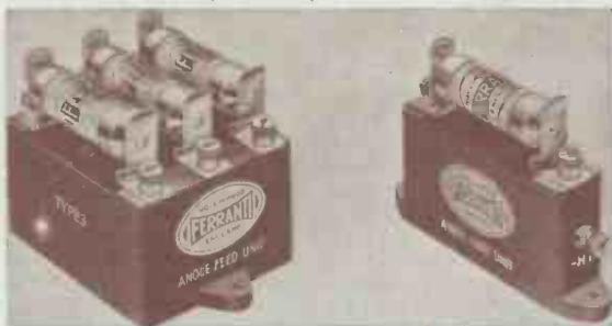
In mains-operated sets it is often necessary to reduce the voltage before application to the valves. This is done by anode resistances, with which are associated fixed by-pass condensers, to prevent low-frequency oscillation or "motor-boating"
