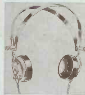
Headphones are still used for commercial work, although not much for broadcast reception. The type illustrated has an adjustment for the magnets
