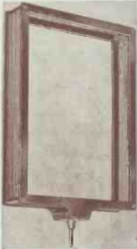
A frame aerial consists of a length of wire wound round a rectangular or other regular-shaped former. It takes the place of an aerial coil in a set and is tuned to the desired wavelength by a variable condenser
