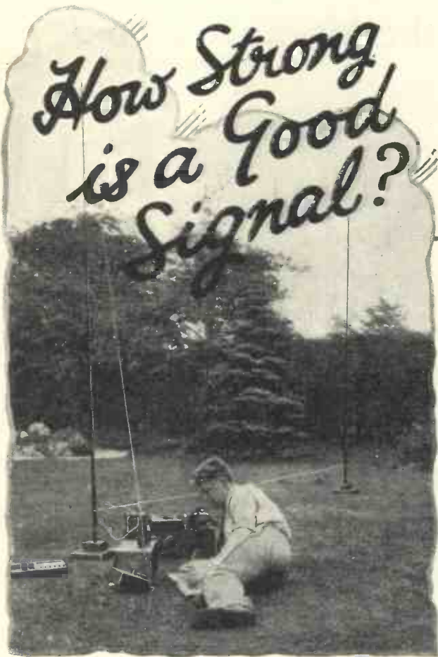
Portable equipment used for check tests on signal strength at the Furzehill Laboratories, Elstree
