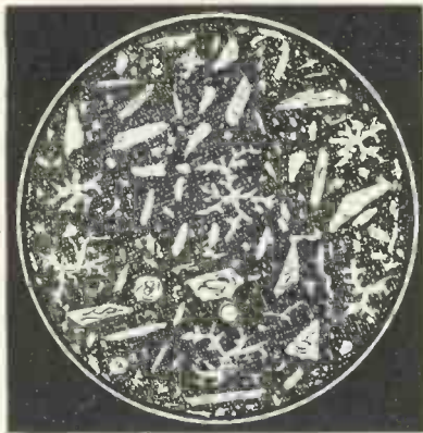
Fig. 1.—Greatly magnified view of the valve mirror (inside), showing its semi-crystalline structure. It consists of sub-limed magnesium
