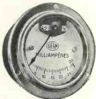
A milliammeter placed in the final output circuit is a check on high-tension current consumption and also detects distortion
